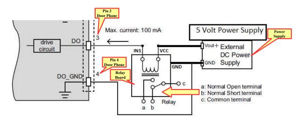
Contacts a, b and c on the Relay Board can be used to operate an external device.
